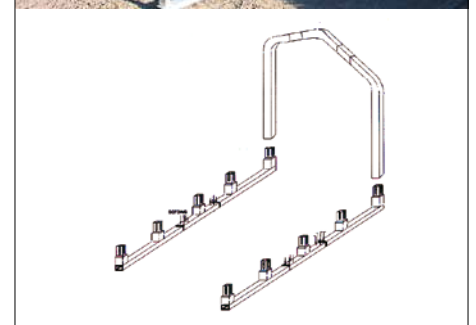
Attach the trusses to base bars: no ladder required. Secure self tappers on all joints.
