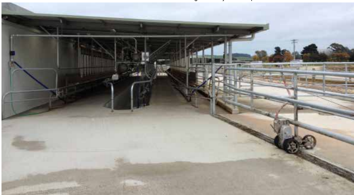
System shown with additional built in yard drain channel.
