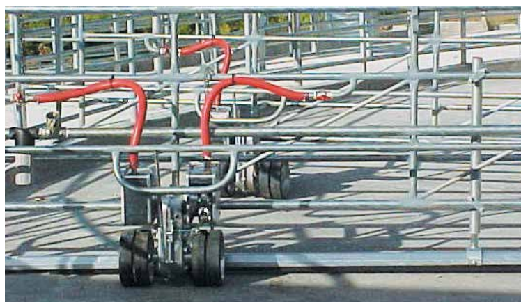
Dual water driven gates.
