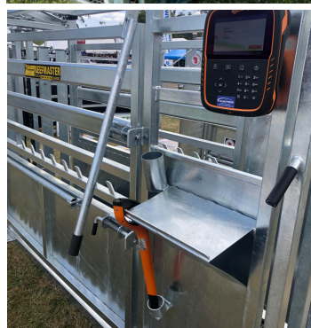
Operation end of the Beefmaster Classic. Monitor, EID wand placement, drink bottle holder, work shelf.
