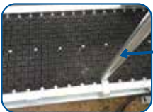
1 SWAY BAR POST Holds the animal while all the gates are open.
