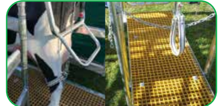
Rear leg hoist from a choice of two lift positions
