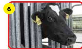
6 The rubber lined yoke and Hydralock system makes the "Dairy Handler" headbail very quiet and light to operate.
