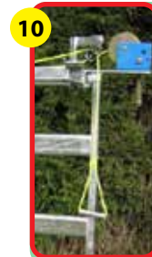
10 The lifting assembly to hoist the leg up. Equipped with quick release for safety.
