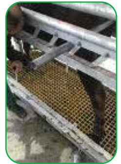
Single side squeeze reduces the width of the unit to get that extra control on any size animal
