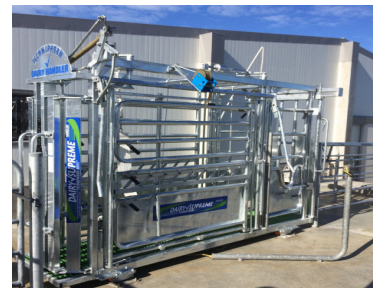
Single side squeeze reduces the width of the unit to get that extra control on any size animal
