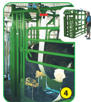
The belly hoist with winch is great for stabilizing the cow and to make sure she stays up
