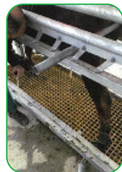
Single side squeeze reduces the width of the unit to get that extra control on any size animal
