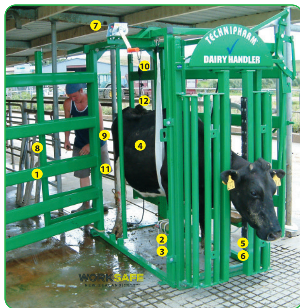
The unique side bar ensures you can open a side gate and yet keep the cow fully side supported - stops her swaying sideways
